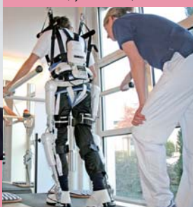
Cyborg-type medical robot HAL ® developed by incorporating 'Cybernetics' (by Prof. Sankai)
